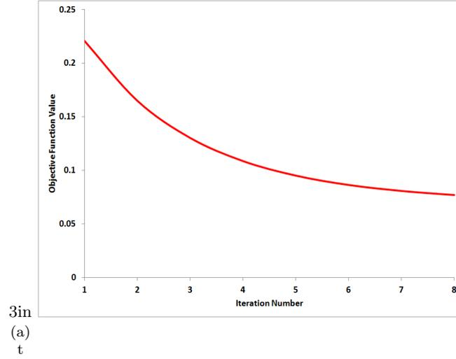
FIG. 5: Variation of the Objective function value with respect to number of iterations of control vector iteration
