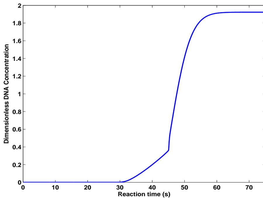
FIG. 2: Optimal DNA concentration profile that was obtained by solving PCR optimal control problem using control vector iteration.
