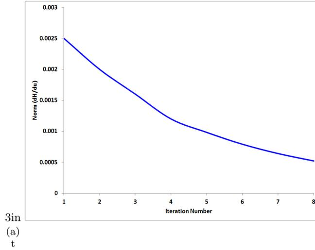
FIG. 4: Variation of the  $\|\frac{dH}{du}(t)\|$  with respect to number of iterations of control vector iteration
