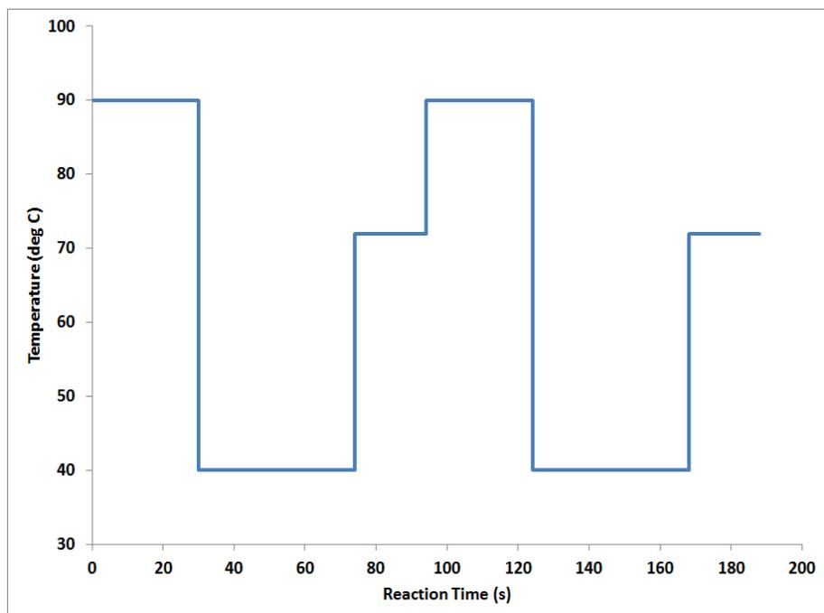
FIG. 8: Optimal temperature profile that minimizes the overall reaction time by cycling switching at the intersection point in Fig. 2.6.
