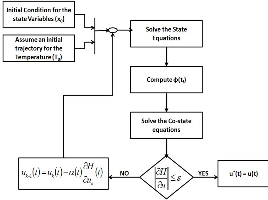
FIG. 1: Control Vector Iteration to solve optimal control problem
